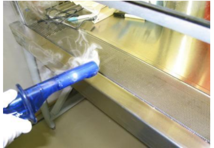
Airflow into the cabinet— As someone walks by
